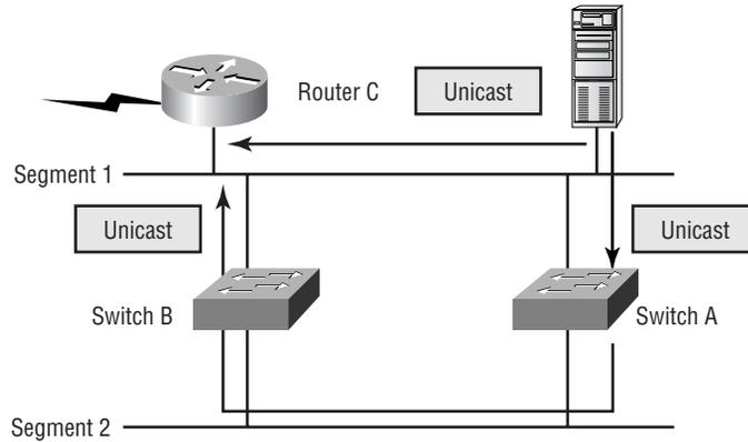
3. The MAC address filter table will be confused about where a device is located since the switch can receive the frame from more than one link. It is possible that the switch can't forward a frame because it is constantly updating the MAC filter table with source hardware address locations. This is called *thrashing* the MAC table.
