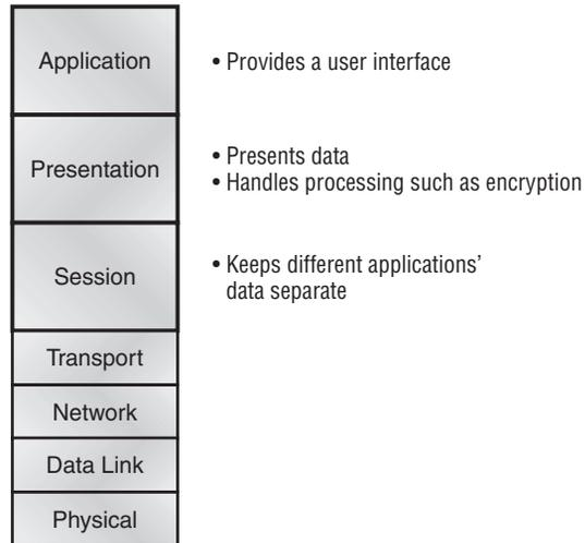
In Figure 1.1, you can see that the user interfaces with the computer at the application layer, and also that the upper layers are responsible for applications communicating between hosts. Remember that none of the upper layers know anything about networking or network addresses. That is the responsibility of the four bottom layers, which are shown in Figure 1.2.
