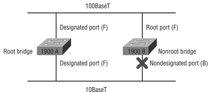
Ports determined to have the lowest-cost path to the root bridge are called designated ports. The other port or ports on the bridge are considered nondesignated and will not send or receive traffic, which is called blocking mode.
