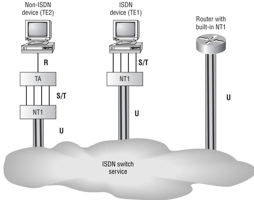
In North America, ISDN uses a two-wire connection into a home or office. That is called a “U” reference point. The NT1 device is used to convert the two-wire connection to a four-wire connection that is used by ISDN phones and terminal adapters (TAs). Most routers can now be purchased with a built-in NT1 (U) interface.
