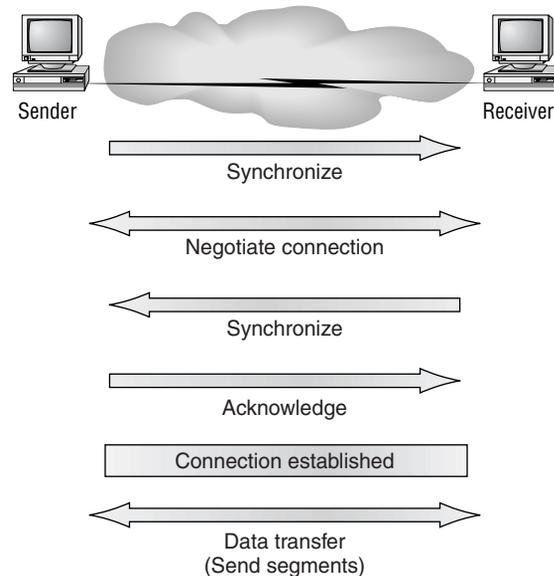
While the information is being transferred between hosts, the two machines periodically check in with each other, communicating through their protocol software to ensure that all is going well and that the data is being received properly.
