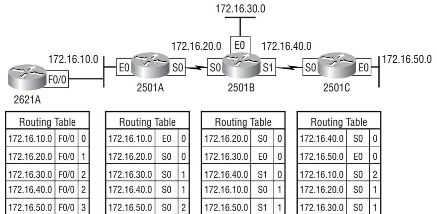
The routing tables in each router keep information regarding the network number, the interface to which the router will send packets out to get to the remote network, and the hop count or metric to the remote network.
