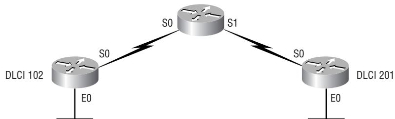
In my seminars I usually use a 2522 router as a frame switch, which provides 10 serial connections. But, since it is possible you may only have some 2501s, I have written this lab to work with three 2501 routers.
