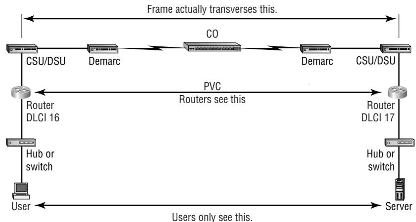
The basic idea behind Frame Relay networks is to allow users to communicate between two DTE devices through DCE devices. The users should not see the difference between connecting to and gathering resources from a local server and a server at a remote site connected with Frame Relay. Chances are this connection will be slower than a 10Mbps Ethernet LAN, but the physical difference in the connection should be transparent to the user.
