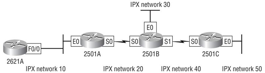
Let's start off by adding the Novell-Ether (802.3) frame type to the internetwork Ethernet networks. Since that is the default encapsulation, the configuration is really simple. The default encapsulation on the serial links is HDLC, and you'll use that as well. HDLC is discussed in Chapter 10.
