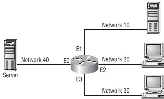
The following configuration is used with Figure 9.2. Interface Ethernet 0 is on Network 40; interface Ethernet 1 is on Network 10; interface Ethernet 2 is on Network 20; interface Ethernet 3 is on Network 30.
