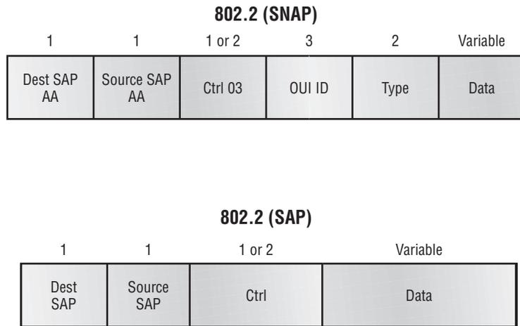
Figure 1.12 shows how the LLC header information is added to the data portion of the frame.
