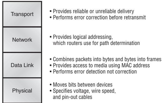
The four bottom layers define how data is transferred through a physical wire or through switches and routers, and how to rebuild a data stream from a transmitting host to a destination host's application.
