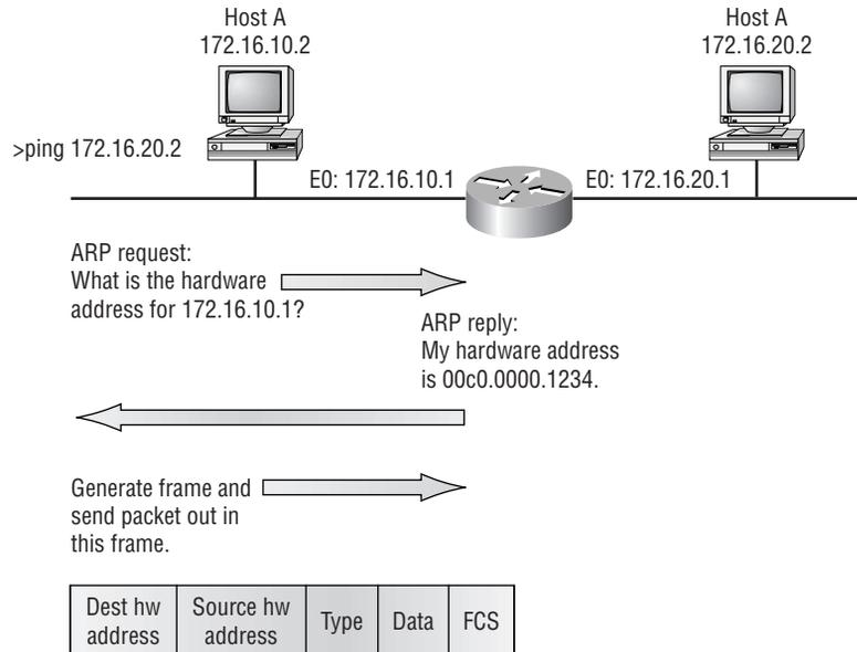
In Figure 5.2, all of the information needed to communicate to the router is shown: the source and destination hardware addresses, the source and destination IP addresses, and finally, the data and the frame's CRC inside the Frame Check Sequence (FCS) field.
