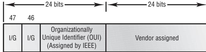
The *Organizationally Unique Identifier (OUI)* is assigned by the IEEE to an organization (24 bits or 3 bytes). The organization, in turn, assigns a globally administered address (24 bits or 3 bytes) that is unique (supposedly) to each and every adapter they manufacture. Notice bit 46. Bit 46 must be 0 if it is a globally assigned bit from the manufacturer and 1 if it is locally administered from the network administrator.
