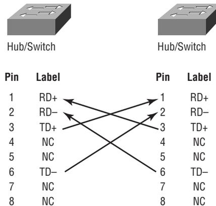
Notice that pin 1 on one side connects to pin 3 on the other side, and pin 2 connects to pin 6 on the opposite end.
