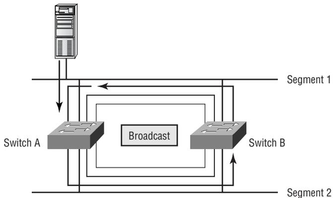
2. A device can receive multiple copies of the same frame since the frame can arrive from different segments at the same time. Figure 2.3 shows how multiple frames can arrive from multiple segments simultaneously.
