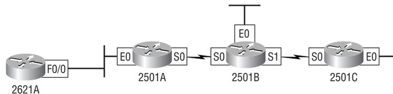
Figure 5.4 shows the three 2500 routers connected via a WAN and the 2621 router connected via the Ethernet network off 2500A. Each router also has an Ethernet network connected.
