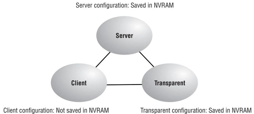
**Server** Is the default for all Catalyst switches. You need at least one server in your VTP domain to propagate VLAN information throughout the domain. The switch must be in server mode to be able to create, add, or delete VLANs in a VTP domain. Changing VTP information must also be done in server mode. Any change made to a switch in server mode is advertised to the entire VTP domain.
