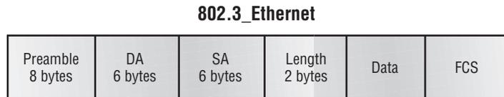
**Destination Address (DA)** This transmits a 48-bit value using the Least Significant Bit (LSB) first. DA is used by receiving stations to determine if an incoming packet is addressed to a particular node. The destination address can be an individual address, or a broadcast or multicast MAC address. Remember that a broadcast is all 1s or Fs in hex and is sent to all devices, whereas a multicast is sent to only a similar subset of nodes on a network.
