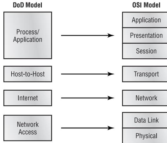
A vast array of protocols combine at the DoD model's *Process/Application layer* to integrate the various activities and duties spanning the focus of the OSI's corresponding top three layers (Application, Presentation, and Session). (We'll be looking closely at those protocols in the next part of this chapter.) The Process/Application layer defines protocols for node-to-node application communication and also controls user-interface specifications.
