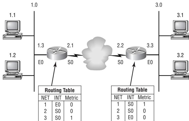
The routing table used in a router includes the following information:
