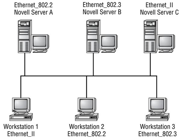
Each frame type in Figure 8.3 has a unique IPX network address. Even though there's a single Ethernet segment, there are three *virtual* IPX networks and, therefore, three unique IPX network addresses. Each network will be broadcast across the internetwork every 60 seconds.
