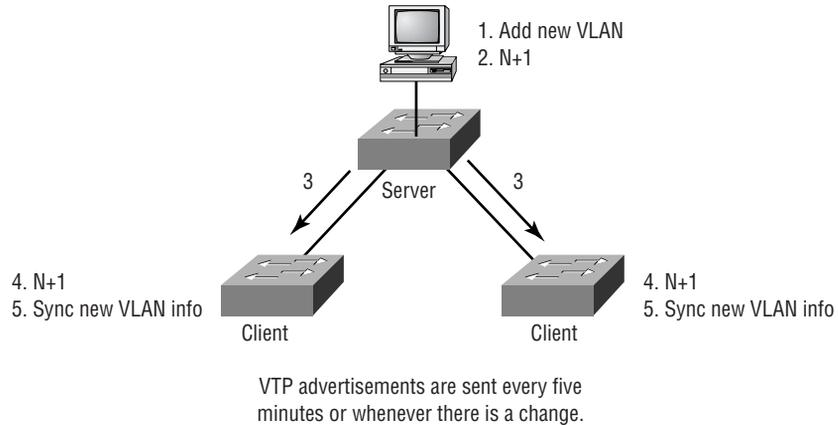
This figure shows a configuration revision number as “N.” As a database is modified, the VTP server increments the revision number by 1. The VTP server then advertises the database with the new configuration revision number. When a switch receives an advertisement that has a higher revision number, it overwrites the database in NVRAM with the new database being advertised.
