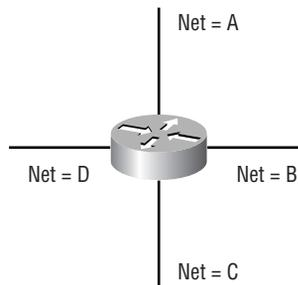
Each network is attached to the router and has its own logical network number. Each node attached to a particular physical network must match that network number to be able to communicate on the internetwork. Now let's look at what a switch accomplishes. Figure 6.3 shows how switches remove the physical boundary.
